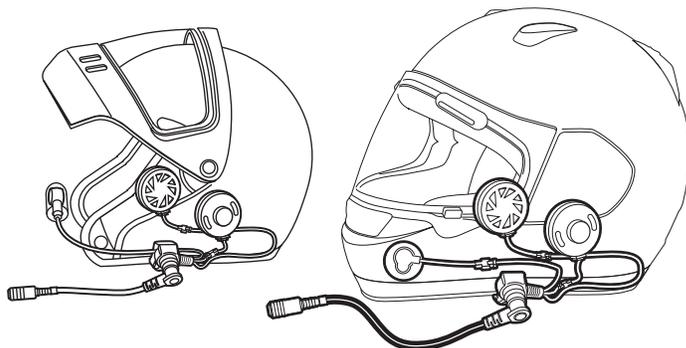
1. Most flip-front & full-face style helmets have cheek pads or a complete nose section that can be removed. Carefully do so at this time, paying special attention so as not to break or damage any of the polystyrene parts.
