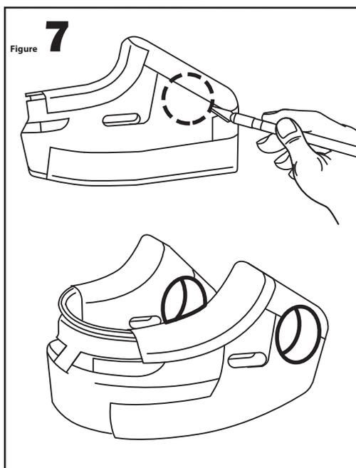
2. Remove the padding material that is installed around the speakers & then using one of the speakers as a guide, mark the area where the circular pieces of styrene will be removed from the back of the ear area of the cheek pad or nose section. **See Figure 7.**
