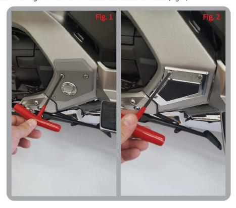
3. Determine correct orientation for the left and right sides of the motorcycle. Install covers using original screws, torque to 5.2 N-m, 3.8 ft-lbs. Do not overtighten. (Fig. 2)
