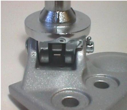
3. Install chrome clevis using pin, washer and cotter key.
