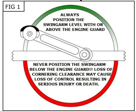
**WARNING** IT IS THE INSTALLERS RESPONSIBILITY TO ENSURE THERE IS SUFFICIENT CORNERING CLEARANCE BEFORE RIDING. ALWAYS POSITION THE SWINGARM EITHER LEVEL WITH, OR ABOVE THE ENGINE GUARD. POSITIONING THE SWINGARM BELOW THE ENGINE GUARD WILL GREATLY DECREASE CORNERING CLEARANCE WHICH MAY CAUSE LOSS OF CONTROL RESULTING IN SERIOUS INJURY OR DEATH.
