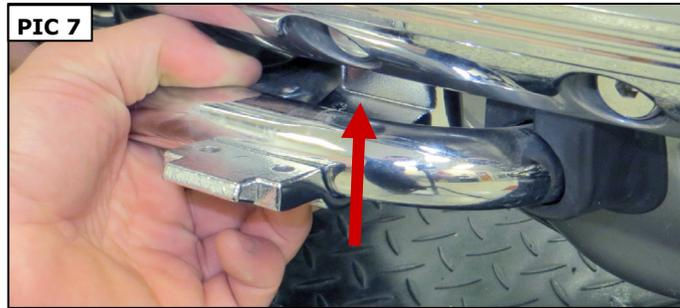
**STEP 7** Refer to **PIC 8**. Position the clutch-side upper clamp-half (separated in **STEP 3**) over the engine guard and align it with the bottom clamp-half. Secure the bottom to the top with the four screws removed in **STEP 3**. **PIC 8**
