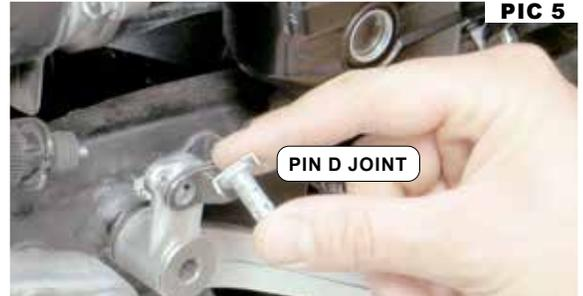
**STEP 5** Unfasten the brake pivot shaft and remove the existing brake lever and flat washer. Set the brake pivot shaft and flat washer aside, they will be reused.
