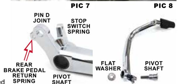
**STEP 9** Align and loosely fasten the brake lever to the motorcycle.
