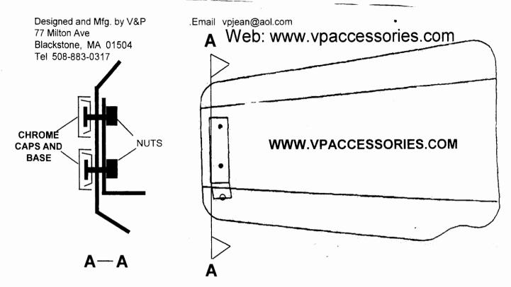
Assemble with hardware shown, with angle on bracket towards the curved knotch on hand warmer. curved knotch is designed to clear top Wind Wing if you have dual wings. If it still touches top wing, your handlebars may have been set too low. To raise the handlebars, remove the key cover and cover on center of handlebars, loosen the four bolts and raise bars till they clear. Tighten bolts and replace covers.
