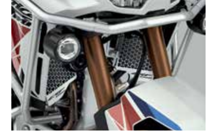
RADIATOR GRILLS 08F71-MKS-E00 Made of stainless steel and displaying a CRF logo, the Radiator Grills increase the African Twin tough image. Their original mesh pattern combines cooling capability with a protection against stone chippings for the radiators.
